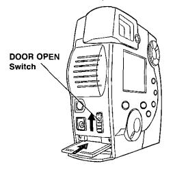
Set POWER OFF before inserting the Memory card.
