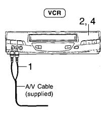
Connect the A/V OUT Terminal on the Camera and the AUDIO IN/VIDEO IN on the VCR or TV using the A/V Cable (supplied).
