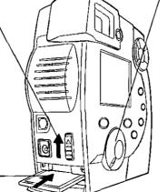
Set POWER Switch to OFF before inserting the Memory card.
