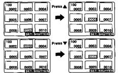
**5** Press SHUTTER to playback the selected image, and to return to Manual Playback.
